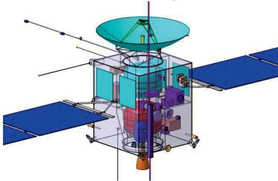
*Figure 2: The JGO Flight System utilizes solar power to operate 10 instruments.*
