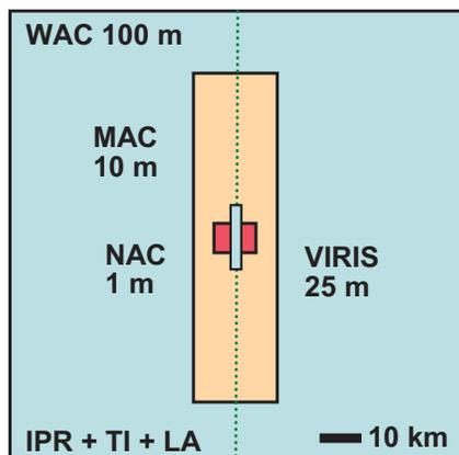
**Figure 3:** *Nested JEO FOVs provide for coordinated targeted observations (resolution/pixel indicated).*
