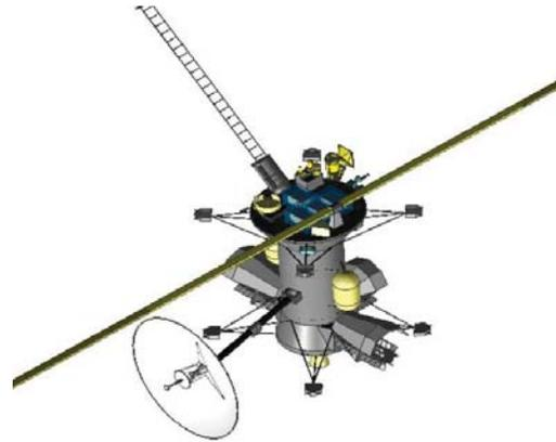
*Figure 3: The JEO Flight System uses radioisotope power to operate 11 instruments.*
